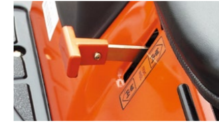
Four Wheel Drive 4WD is standard on the CS2610 tractor and a single lever engages the 4WD.
