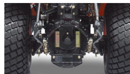
Rear PTO and 3-Point Hitch The rear PTO and high capacity three point hitch can accommodate a variety of implements and attachments. The flip up PTO guard ensures easy implement attachment. The bent lower link assist with easy implement installation.
