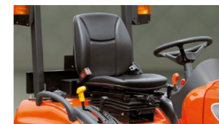
Ergonomic Operator Station The ergonomically designed work station places operator controls within easy reach to enjoy a comfortable and smooth ride. The retractable seat belt is included for safety.
