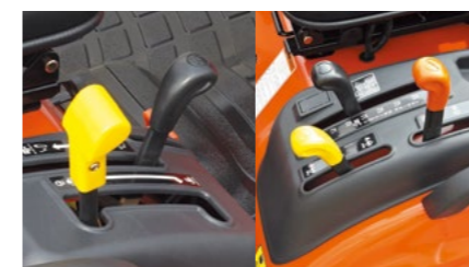
Left Hand Lever Controls The HST with HI-LO range lever allows the tractor to overcome a wide range of load tasks. The rear PTO and mid PTO can be controlled separately or together with a simple in-line shifting lever. The height adjustment lever allows the operator to control the mid-mount mower grass cutting height easily.
