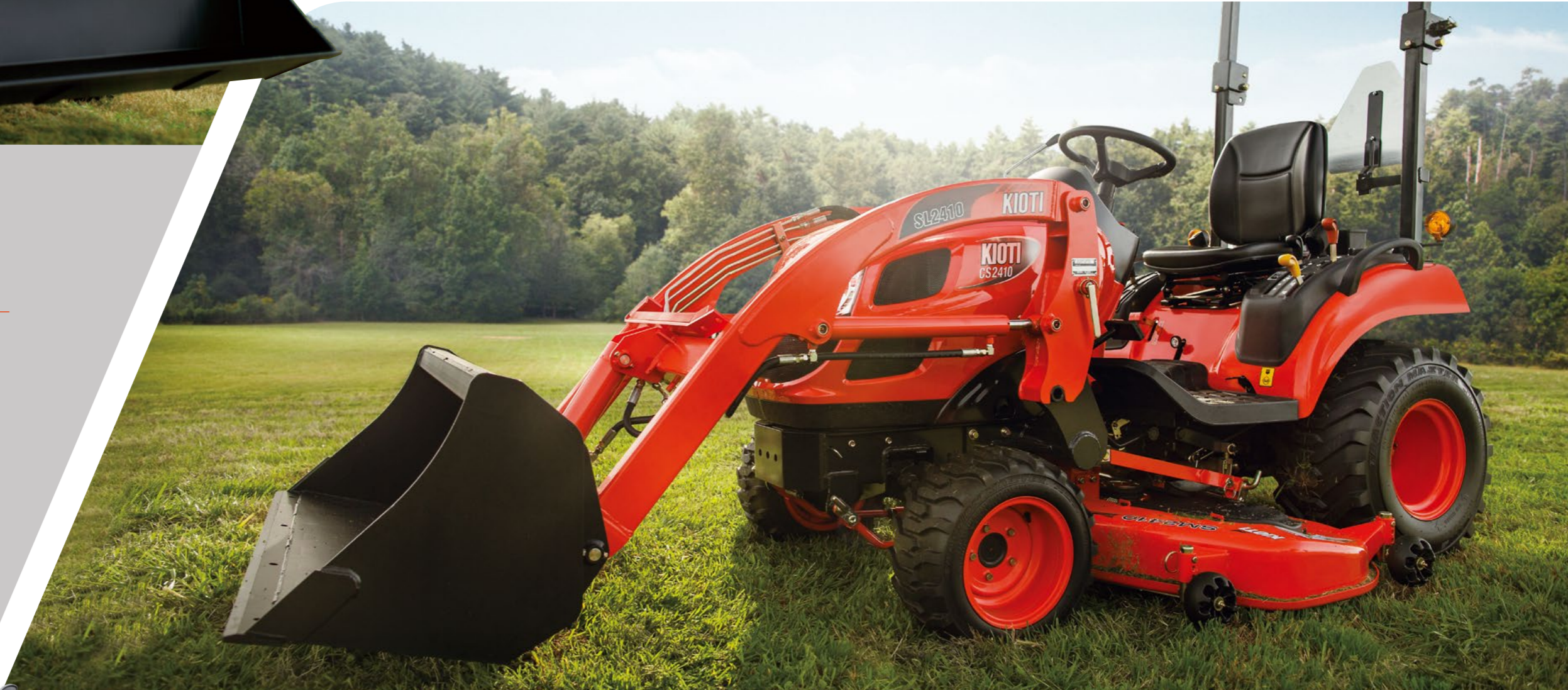
Four Wheel Drive 4WD is standard on the CS2610 tractor and a single lever engages the 4WD.
