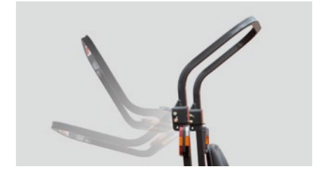
Foldable ROPS The standard fold-down roll bar makes it quick and easy to maneuver in low clearance areas.
