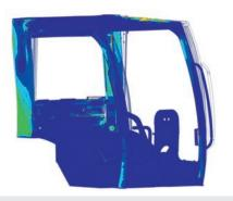
ROPS-FOPS approved cab designed with safety cell to prevent deformation in the event of vehicle overturn or a heavy load falling on the cab.
