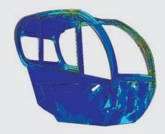
ROPS-FOPS approved cab designed with safety cell to prevent deformation in the event of vehicle overturn or a heavy load falling on the cab.
